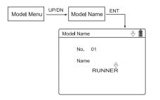
Press UP or DN button to select the characters which need to be changed, press R or L to change the characters. Name model "RUNNER". Press EXT to return to the "Model Menu".
